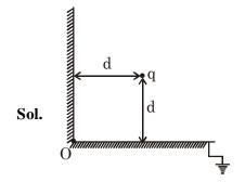
By method of image, the given arrangement is equivalent to
